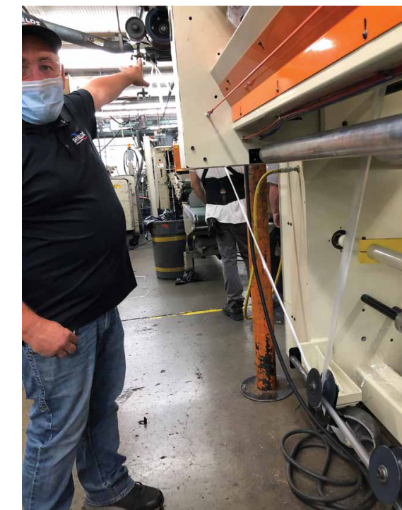
At Novolex's Shields facility in Yakima, Wash., an employee shows how trim scrap is captured and re-inserted into the manufacturing process.
